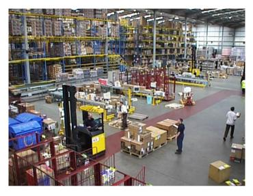
Operates Monday – Friday, 6am-8pm. With a small night shift and capacity to operate 24hr / 7days. Storage is arranged logically such that fastest moving items are within easy access areas. All locations within the warehouse are bar-coded including floor areas. There is a mezzanine forward pick area, which is used for the 200 fastest moving line items.
